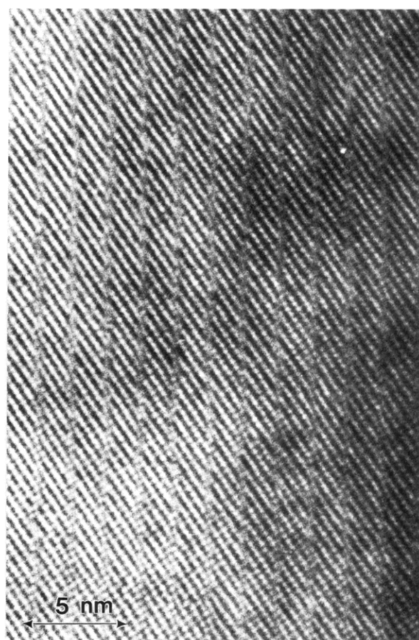
Figure 2. Electron diffraction pattern (a) and corresponding lattice image (b) for \text{Ba}_3\text{Bi}_2\text{BaO}_9 showing the commensurate superlattice and the periodic antiphase boundaries. The Ba/Bi order is not apparent in the lattice image. However, lattice image simulations show that for most imaging conditions, the contrast arising from the cation ordering is expected to be weak.
